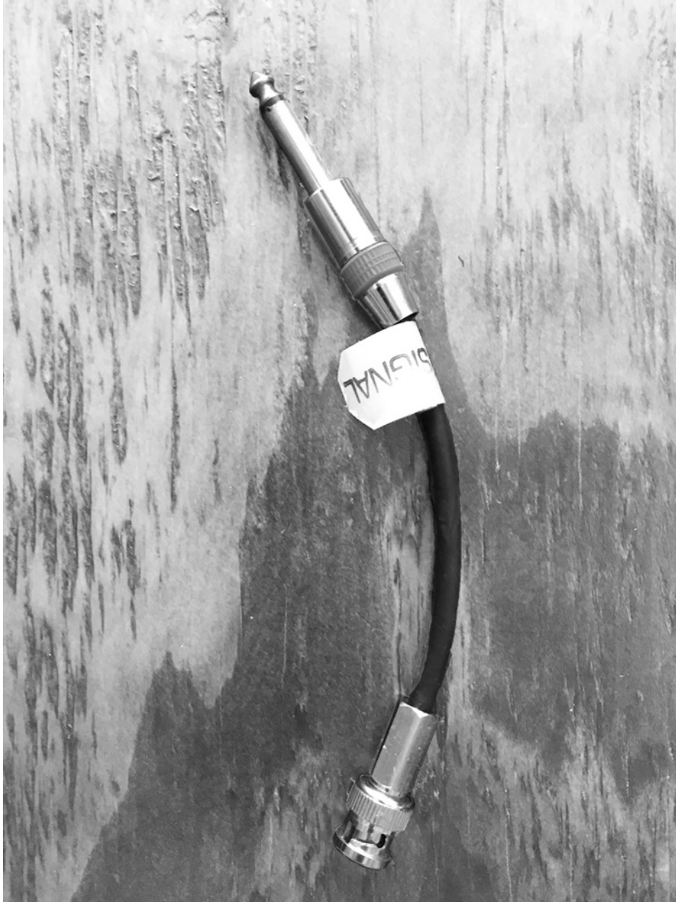
Figure 5: vaudio signal (Ben Baker-Smith and Evan Kühl) album release as cable, 1/4" to BNC. Photo © Ben Baker-Smith and Evan Kühl, used by permission.
